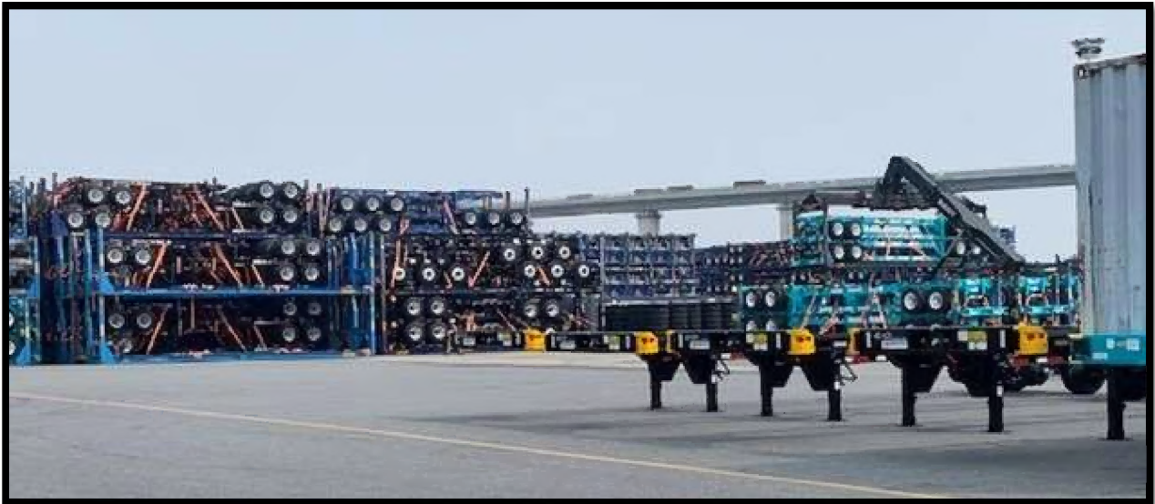
Figure 4: Example of Chassis Prepared for Export in Flat Racks
